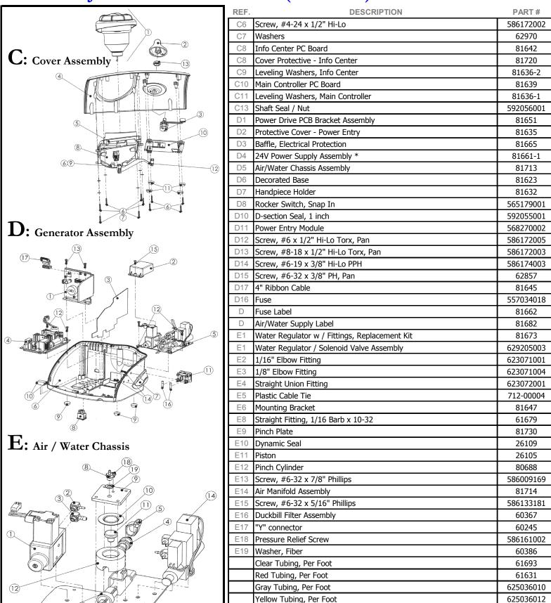
\* NOTE: When replacing p/n #81661-1 24V Power Supply Assembly, be advised to also order #81648-1 and #81649-1 Wire Harness assemblies when upgrading the power supply to the current Meanwell configuration.
