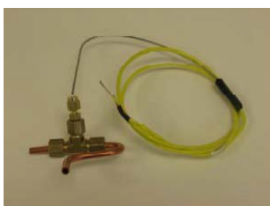
Validation Thermocouple #01-108983S
